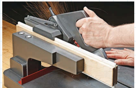
▲ Resin slides mounted in the rail accept the carriage and handle assembly, allowing the grinder to slide back and forth.
