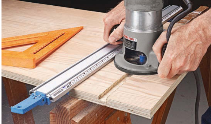
◀ A clamp-on straightedge ensures precise results when routing dados. You'll need to account for the offset between the bit and the straightedge.
