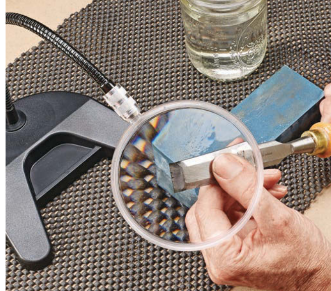
▲ This benchtop magnifier features an acrylic lens and a flexible gooseneck that is easy to adjust. The weighted base keeps the magnifier from tipping over when moved around.
