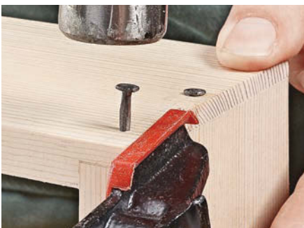
▲ In order to prevent the short grain section from splitting out, clamp across the joint to support the end of the workpiece.
