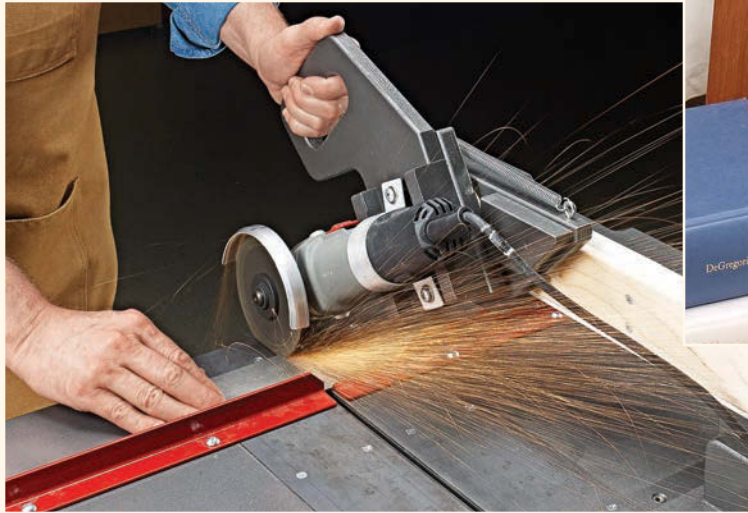
▲ Cutoff Grinder. Give your hacksaw a rest by building this sliding cutoff grinder. It uses an inexpensive angle grinder and an abrasive wheel to make quick work of cutting metal stock to length. You'll find all the details on page 34.
