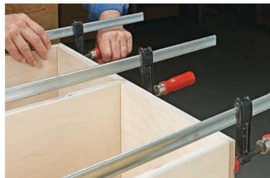
▲ Dados and rabbets simplify case assembly, ensuring that parts are square and aligned as you add glue and clamps.
