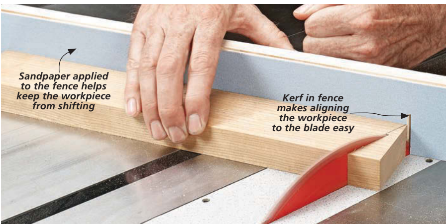
▲ A long plywood auxiliary fence on the miter gauge provides a larger support surface to guide a workpiece for a steady cut. The fence should extend beyond the blade on the waste side of the cut so that you can safely push the waste piece away from the back of the blade.
