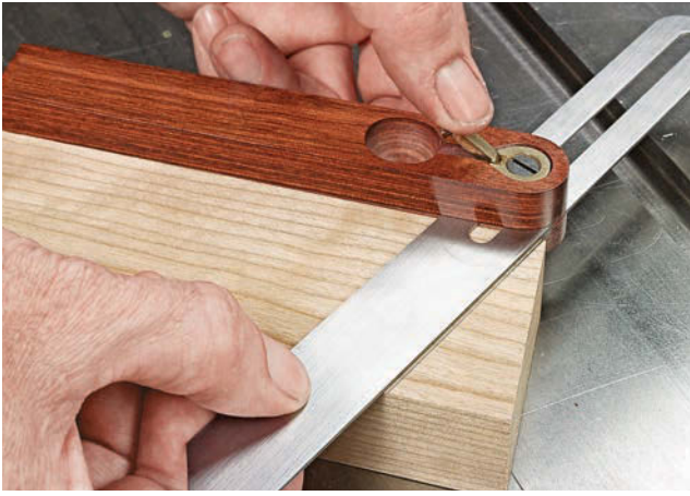
▲ Lay out the starting and ending points of the angle directly on a workpiece. Then set the blade of a bevel gauge to line up with the marks. Use this piece as a setup gauge.
