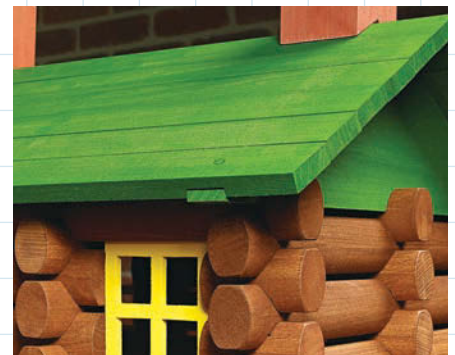
▲ The "starter" slat for the roof fits over short dowels in the gables to support the remainder of the roof.
