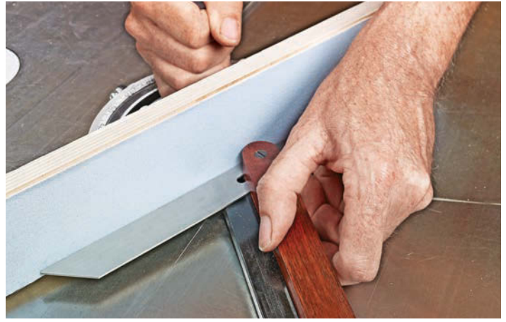
▲ Hold the stock of the bevel gauge against the bar of the miter gauge. Then rotate the miter gauge fence until it aligns with the blade of the bevel gauge. This will ensure consistent cuts.
