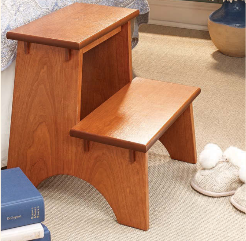
▲ Step Stool. Tapered sides and through mortise and tenon joints give this step stool a leg up on the competition. For a small project, it packs a big woodworking punch. Learn more about building it by turning to page 28.
