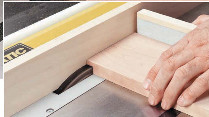
▲ A dado blade allows you to fine-tune the width of a dado or groove for a perfect fit with a mating board. For a rabbet, you can accomplish this by burying the blade in an auxiliary fence (inset).
