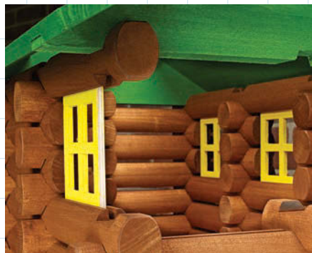
▲ Windows and doors fit into grooves cut into the logs. The window openings are cut on a scroll saw.
