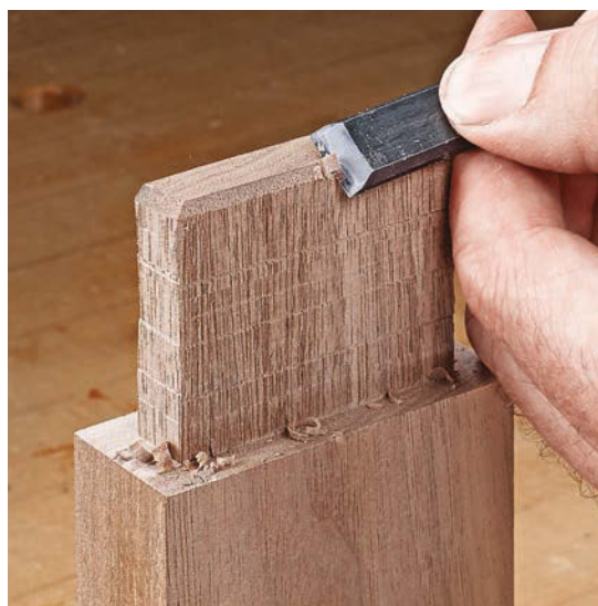
▲ A paring chisel excels at making fine cuts where appearance counts, such as a through tenon. It's easy to control the cutting action for consistent results.
