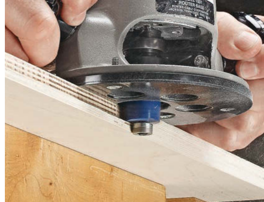
▲ A rabbeting bit has a bearing that rides along the end or edge of a workpiece, guiding the bit as it cuts the rabbet.
