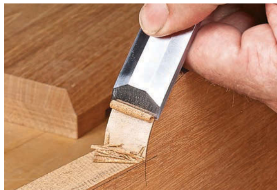
▲ Making controlled cuts to bring a curve to final shape is best done with a paring chisel. Once you get the hang of it, you can create thin curls for a smooth surface.
