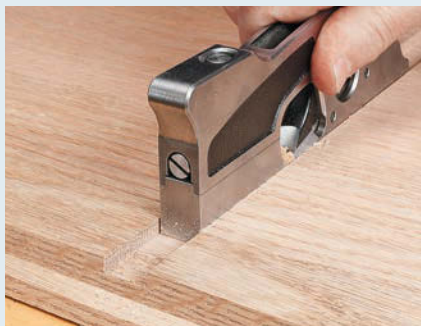
▲ A few quick swipes with a shoulder plane remove ridges and leave a smooth, flat-bottomed dado.
