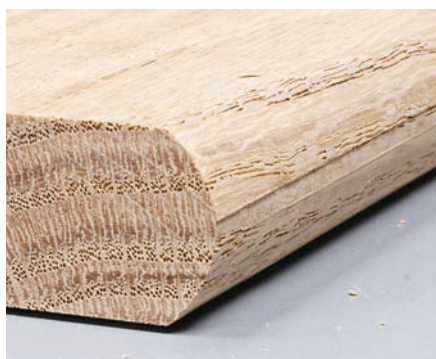
▲ Cutting a bullnose in two passes with a roundover bit can produce a ridge in the middle, but it's easy to sand away.
