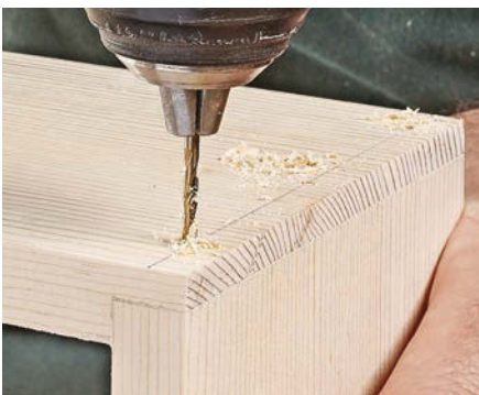
▲ Driving nails near the end of a workpiece may cause a split. So drilling a pilot hole after assembly is a must.
