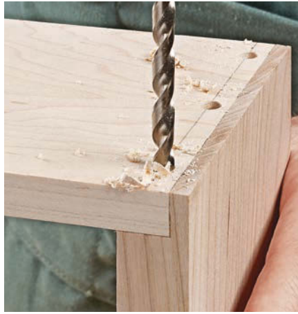
▲ Wait until after the glue dries before drilling holes for dowels. This prevents the parts from shifting out of alignment.
