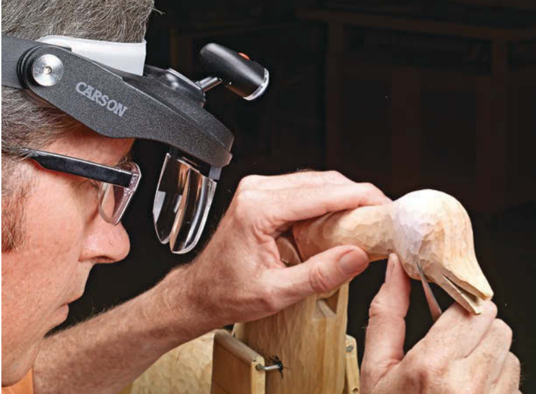
▲ Head-mounted magnifiers, like the Carson Pro MagniVisor , are perfect for tasks where you'll be continually shifting your focus. This is a time-saving advantage when working on different areas of a sizable project.
