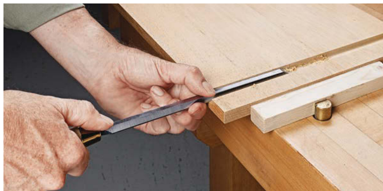
▲ The longer length of a paring chisel can work to your advantage. The lower bevel angle and flat back work to push through high spots to create a flat dado of consistent depth as you lean into the cut with your body.
