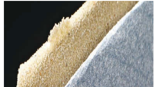
▲ The rigid adhesives used in some inexpensive sandpapers (left) tend to crack and flake off when the paper is folded, as shown above.
