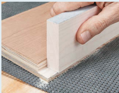
▲ If you don't have a shoulder plane, attach self-adhesive sandpaper to the edge of a scrap block to smooth the joint.
