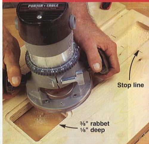
Rout a ⅜" rabbet ⅛" deep along the edges of the 3½"x3½" cutout and the edges of the 2½"-wide channel, stopping 3" from its end.
