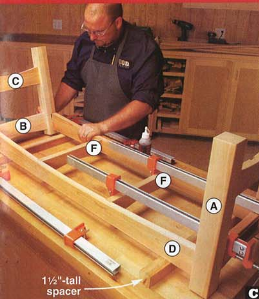
With the seat support assembly (D/F) on 1 1/2"-tall spacers, glue and clamp the end assemblies (A/B/C) to the front/back rails (D).
