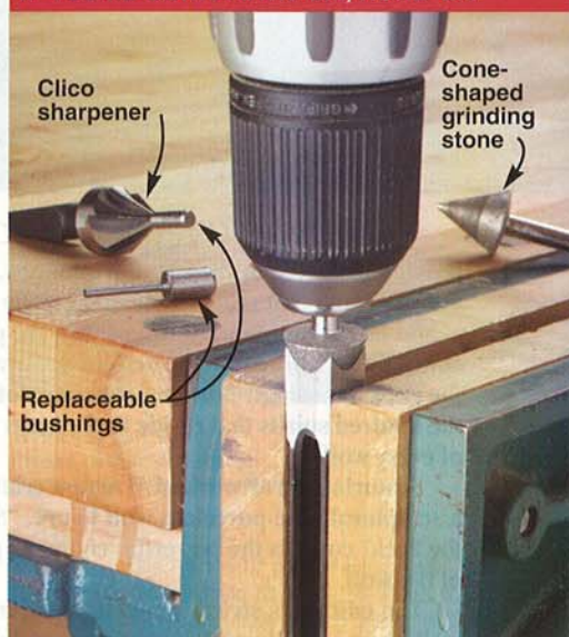
Cone-shaped grinding wheels put a sharp edge on the business end of a hollow mortise chisel held in a vise. The fluted Clico sharpener (at left in photo) works only on that brand of chisels.
