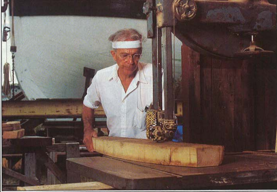
Clete Plamondon shapes a 3"-thick piece of white oak at the old bandsaw.
