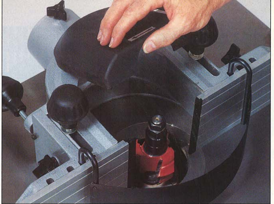
Seco's fence includes a hinged lid and a steel safety guard that mounts in holes in the top of the fence halves.
