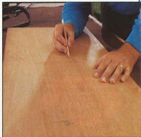
The foundation of a perfect finish is the sanding. With a pencil, Marlen marks sanding scratches to be removed.
