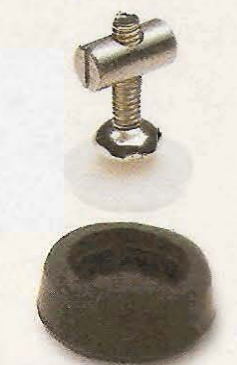
▲ Clamp Pad. To make the clamp pad, thread a leg leveler into a barrel nut. Then cut off the end of a rubber crutch tip and slip it over the leg leveler.
