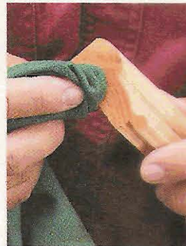
▲ Smooth Cutting. Dampening the end grain with a wet cloth makes it easier for the plane to slice through the wood without tearing the fibers.
