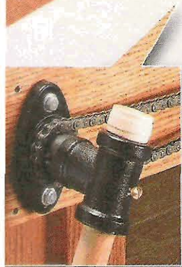
▲ With the vise cover removed, you can see the chain-drive mechanism that operates the vise.
