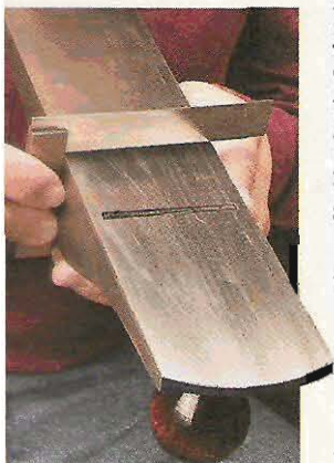
▲ Check for Square. To get good results, the sides of your plane need to be square with the sole.
