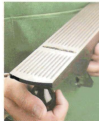
▲ Corrugated Sole. Shallow grooves milled into the sole of this plane are designed to decrease friction while planing.
