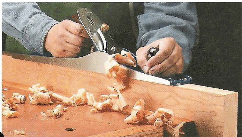
▲ Jointer Plane. The long sole of this #7 jointer plane helps to level the high spots and create a smooth, straight edge on the workpiece. This is important for getting strong, tight-fitting joints when edge-gluing boards.
