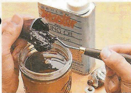
▲ Mixing the Finish. Mixing three tablespoons of Van Dyke brown artist's oil color with a quart of finish gives the workbench a nice, antique oak look.
