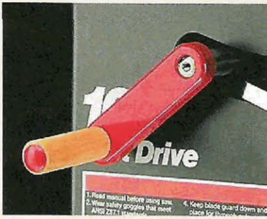
▲ This shop-made crank provides plenty of leverage when adjusting tools and accessories.
