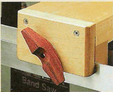
▲ Besides providing finger clearance, a shop-made wing nut allows you to exert plenty of torque.
