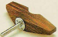
You can make a threaded stud by epoxying a cutoff bolt in the T-nut.
