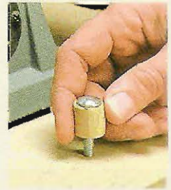
This simple shop-made pin prevents the tool being used from vibrating off the stand.
