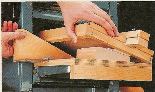
1 Use a scrap with the desired bevel marked on the end to establish the angle of the table. Then slide in the table supports and lock them in place.
