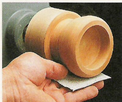
A. Sanding. Hold the sanding pad along the bottom of the workpiece and sand with the rotation.
