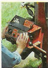
8 As the blade slices through the log (left), the feed rate is controlled by the sawyer (center). A gauge (right) helps determine the thickness of the board.
