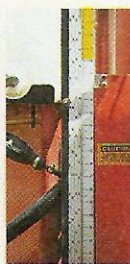
8 As the blade slices through the log (left), the feed rate is controlled by the sawyer (center). A gauge (right) helps determine the thickness of the board.
