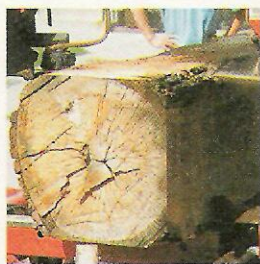
8 As the blade slices through the log (left), the feed rate is controlled by the sawyer (center). A gauge (right) helps determine the thickness of the board.
