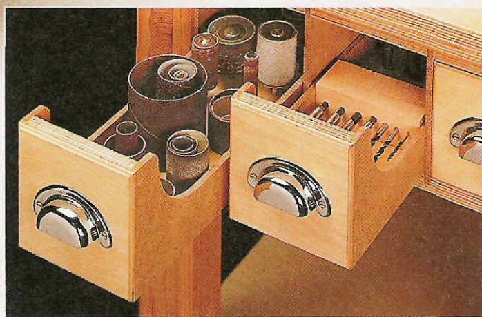
B. Pull-Out Trays. Three pull-out trays provide storage for drill bits and accessories. Scooped sides make it easy to remove bits. And custom bit holders keep them organized.
